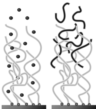
Figure 1. Schematic depiction of the penetration of polymer brushes by low (left) and high (right) molecular weight molecules.
